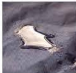
Weather and Water Resistant Generation II Nylon with 3 layers of PU coating underneath.
